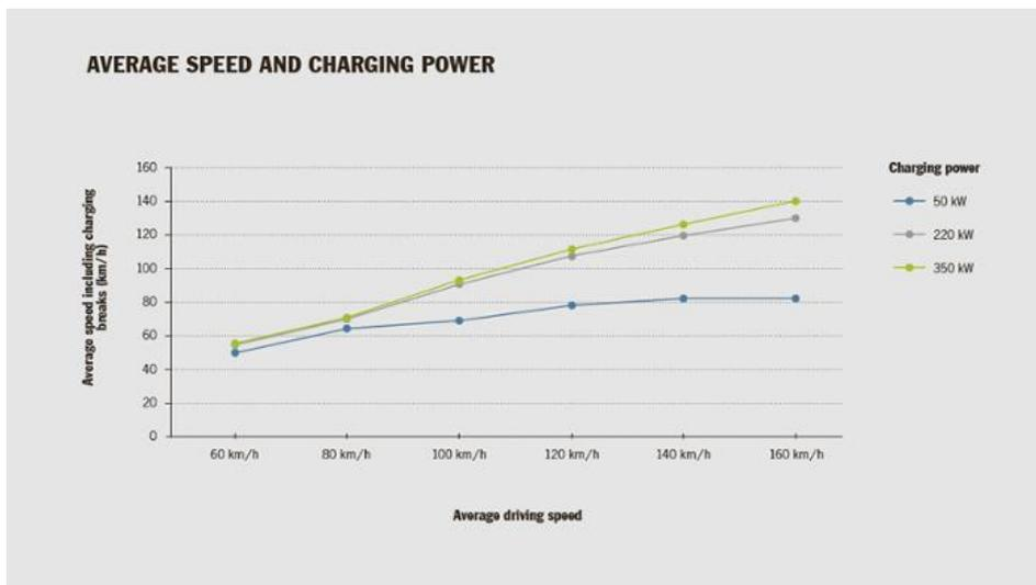
**Figure 2: Achievable average speed in relation to the charging power**
