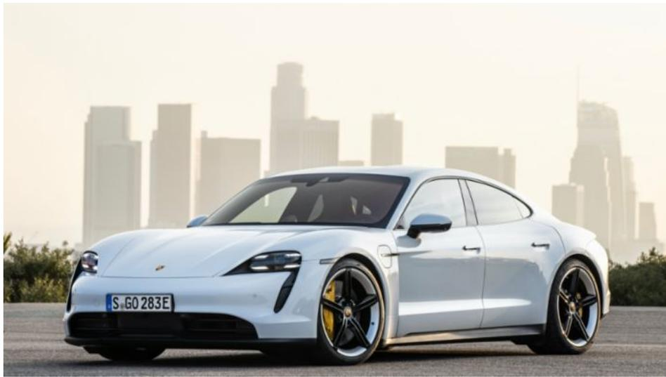
Innovations in the electric Porsche recognised by the scientists at CAM include its 800-volt architecture, two-speed transmission on the rear axle, high recuperative power of up to 265 kW and best cd value in the segment (from 0.22).
