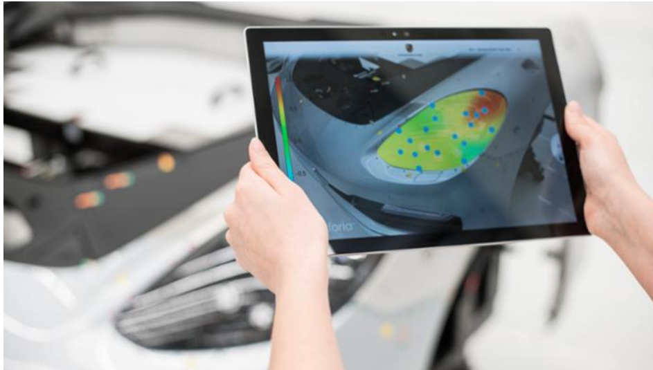
The tablet app superimposes the flaws found during the test over an image of the vehicle
