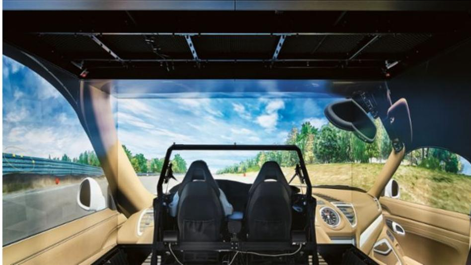
The simulator enables highly precise tests of the interaction between the driver and the technology in practically every stage of the creation of new vehicles, systems and functions. The application spectrum ranges from the display of virtual reality within and outside of the vehicle to tests with complete vehicles.
