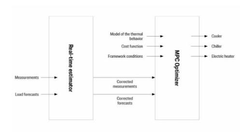
The real-time estimator (RTE) predicts the thermal load that the vehicle will generate in the future (for example, in 40 minutes). To do this, it combines the current state of the vehicle, externally supplied load predictions, and a model of the vehicle's behavior. The MPC Optimizer (model predictive control) controls the heating and cooling system, taking into account not only RTE calculations but also comfort and efficiency requirements (expressed by the cost function and constraints)
