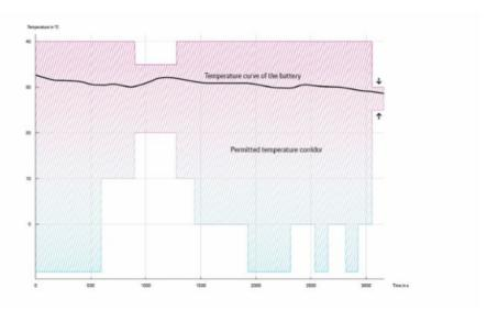
The black curve shows how the battery temperature changes over time. On arrival at the charging station, it is precisely in the optimal range between 25 and 30 °C thanks to predictive thermal management. So the battery can be recharged at maximum power in just a few minutes
