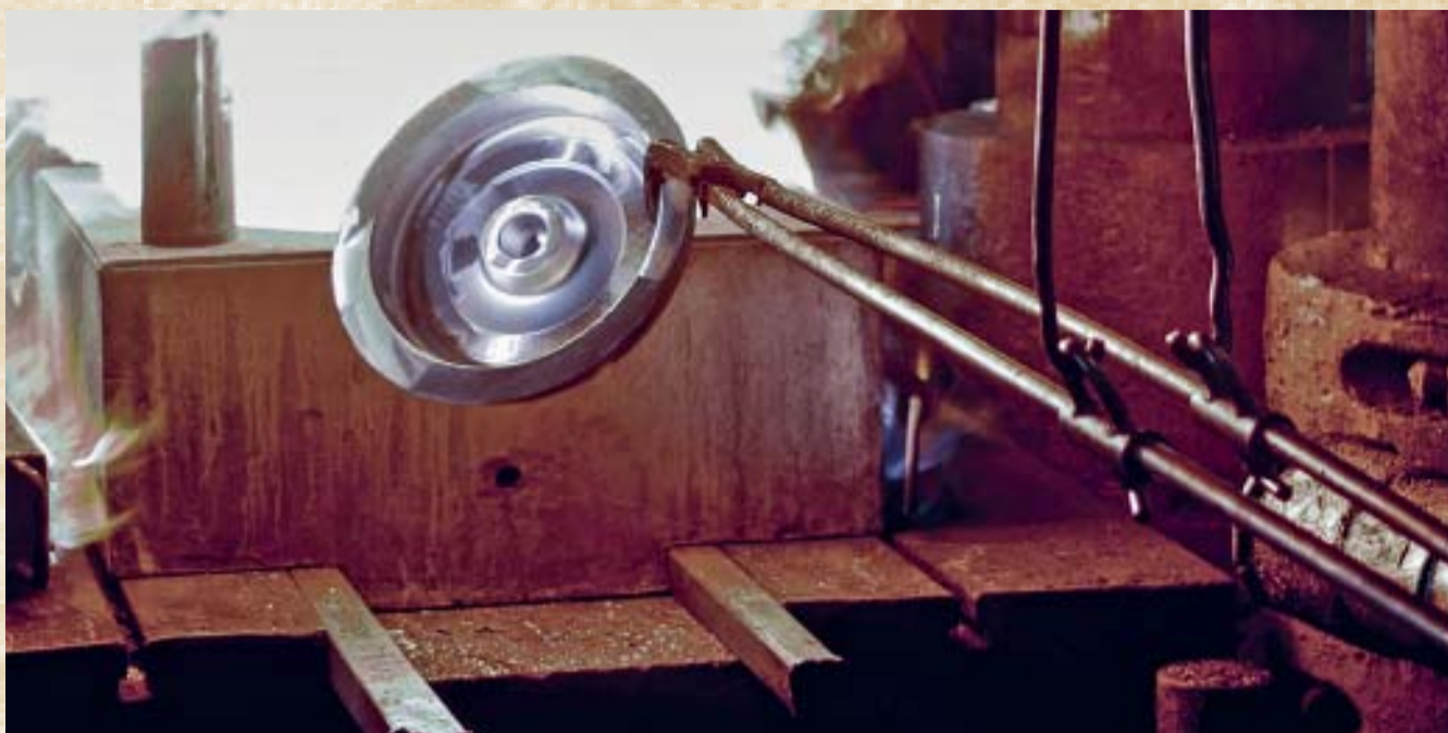
A forged aluminium blank is the starting point for forming the drum in a hot-rolling process.
