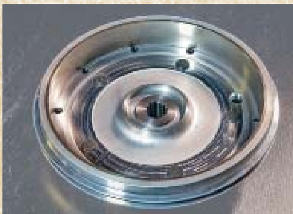
Brake drum 356, front axle Part no. 356 41023 356 A (1950–1959)
