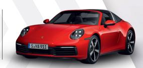
Front gauge: 1,591 mm Rear gauge: 1,557 mm
