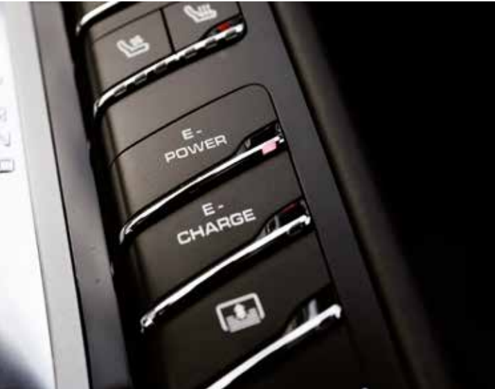
At the push of a button: In "E-Power," the Panamera S E-Hybrid runs solely on electricity, and in "E-Charge," it recharges the lithium-ion battery while driving.
