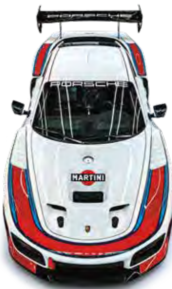
Like its historical predecessor, large parts of the body were replaced or supplemented by carbon-fiber reinforced (CFRP) parts
