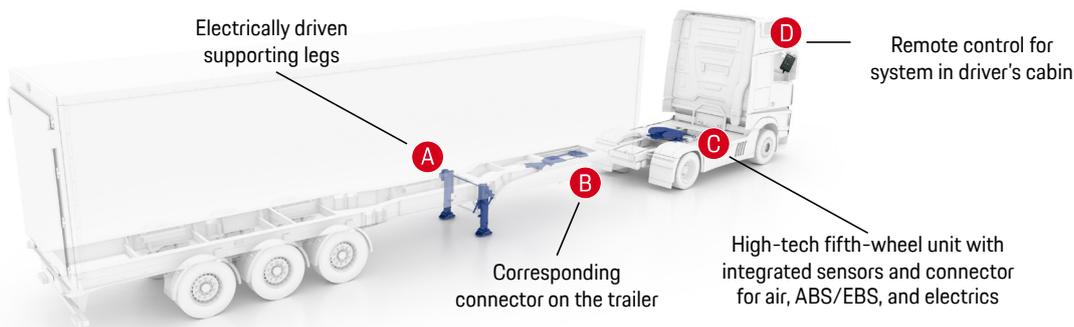
Figure 6. Illustration of four technological components enabling automated trailer coupling. Source: JOST
